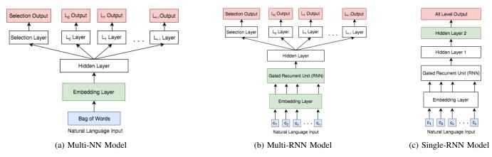
Fig. 2: Model architectures for all three sets of deep neural network models. In blue are the network inputs, and in red are the network outputs. Going left to right, the green denotes significant structural differences between models.
